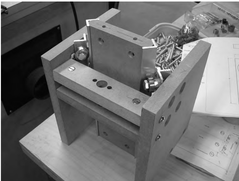
Figure 16-12. Use bolts and cross dowels to secure Part N horizontally between Parts W and X.
