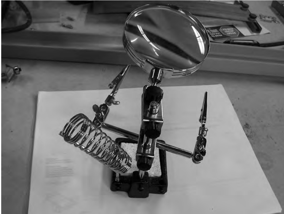
Figure 2-6. A third-hand clamp is very useful when soldering.
