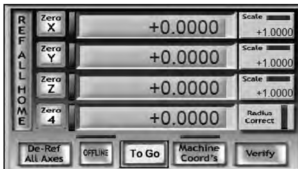
Figure 18-9. Set all the motors' starting position values to zero before testing.
