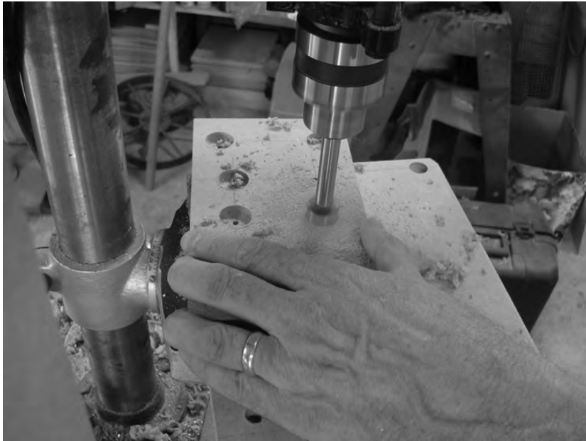
Figure 13-6. Drilling the counterbored holes in Part C
