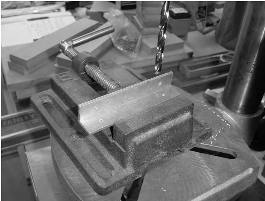
Figure 4-8. Four pilot holes drilled into a rail
