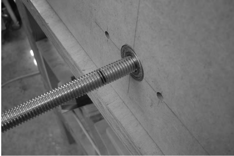
Figure 9-9. Mark an extra 1" of lead screw on both ends of the table and cut.
