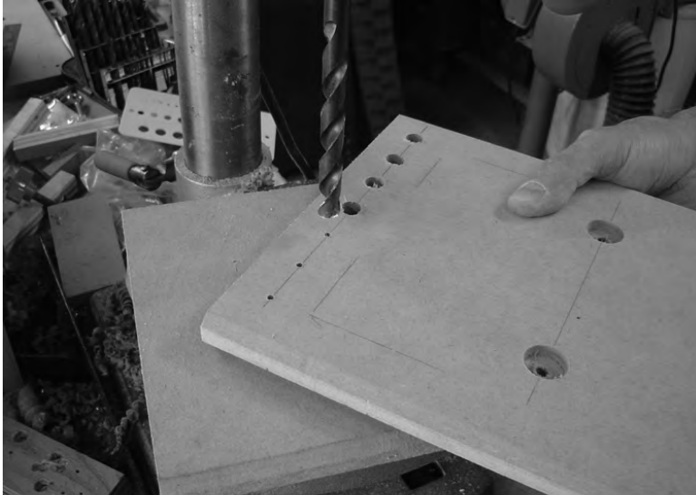
Figure 12-9. Drill the holes for the cross dowels that will be inserted into Part O.
