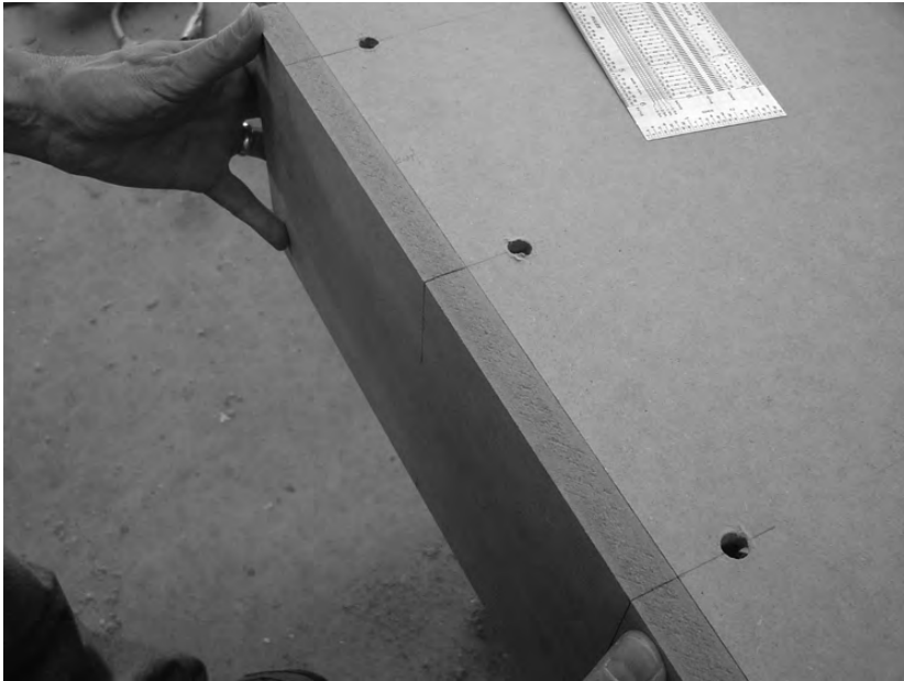
Figure 8-10. Make certain the legs are centered properly.
