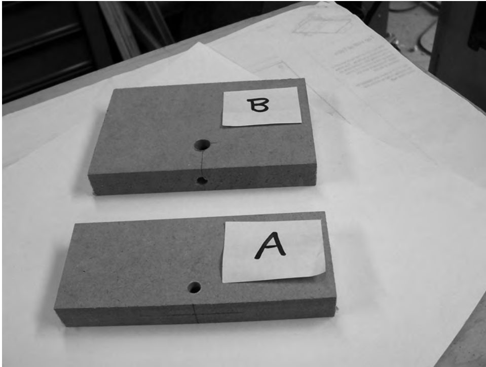
Figure 5-3. Holes will be drilled in each piece of MDF—one hole in Part A and two holes in Part B.
