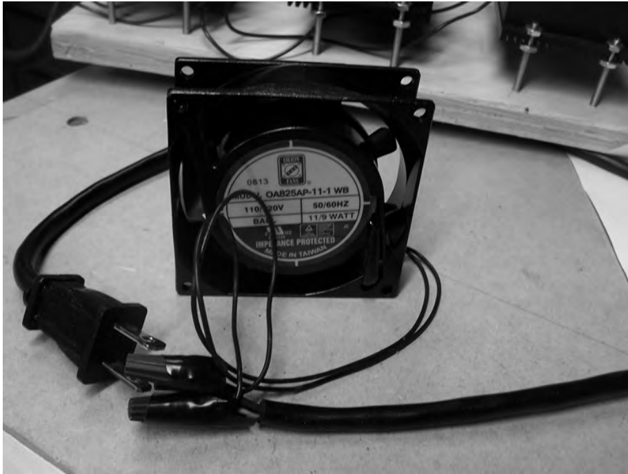
Figure 6-27. The fan will help keep your stepper motor drivers cool.
